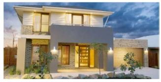
Figure 3: Face brickwork permitted however must be used in a combination with other materials such as painted render
